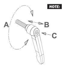
To adjust, tilt pull handle out (B) and rotate counter clockwise (A), release and tighten. If needed, use  $\frac{1}{8}$ " hex head wrench for adjustment (C)
