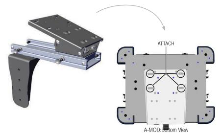
3. Pull the rear knob to release and move the top assembly. Slide it forward to the front locating knob and it will automatically lock in position. From this point you will be able to mount A-MOD Desktop/docking equipment to the top plate via holes and slots from the underside with provided ¼"-20 bolts and washers.
