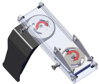
4. The swivel tension to the Motion Arm and Tilt/Swivel Assembly is set at the factory. This can be adjusted by loosening and/or tightening the (3) <sup>1</sup>/<sub>4</sub>"-20 nuts at each location. Use a <sup>7</sup>/<sub>16"</sub> wrench to stabilize the nut and a <sup>5</sup>/<sub>32"</sub> T-handle hex key to turn the bolt.
