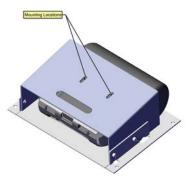
Flip the faceplate and printer over and tighten two small screws on the bottom of the printer/faceplate to secure the printer.
