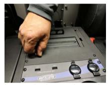
Loosen knob to release the printer faceplate from its secure position.
