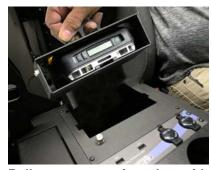
Pull up to remove faceplate with printer from console when the paper roll needs changing.
