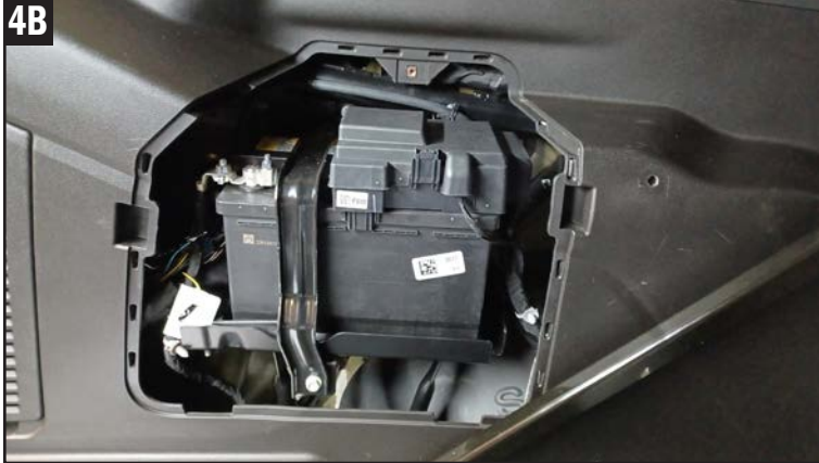
4 Remove the screw and pop loose to remove the battery cover. Tool Required 7 MM Socket.
