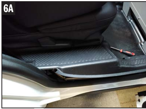
6 · Pop loose the (2) press in pins holding the panel to the lower seat skirt fabric, remove trim section. · Fold the rear seats down and pull the rubber door seal away from the "C-Pillar" side panel.
