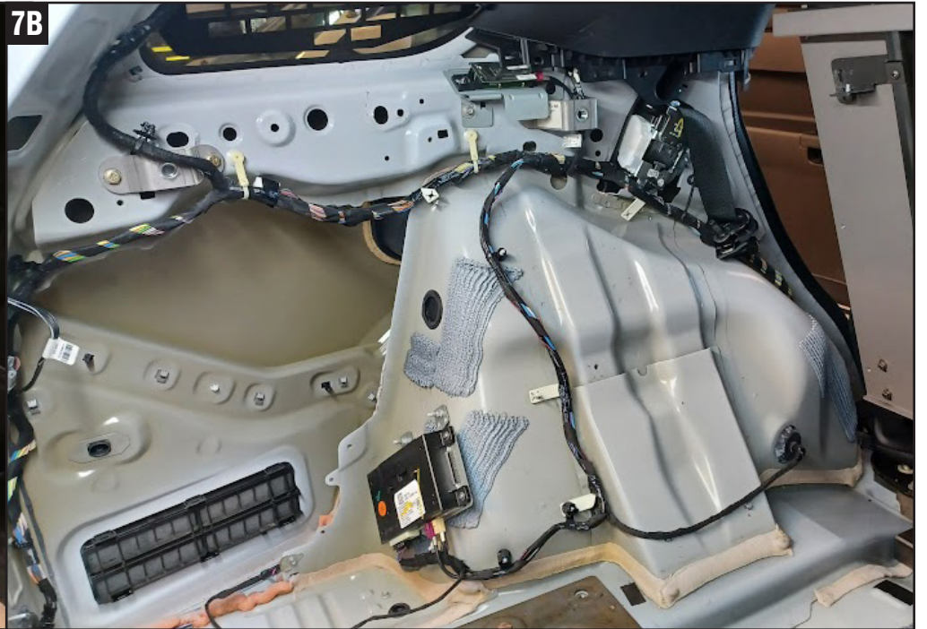
7 Starting from the cargo area, pop loose the upper panel while moving forward to the rear seat area. Once loose, remove from vehicle.
