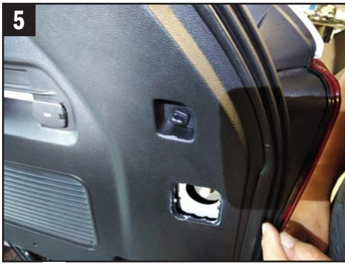
5 Unscrew the accessory hatch cover pin from the rear of the cargo upper trim.
