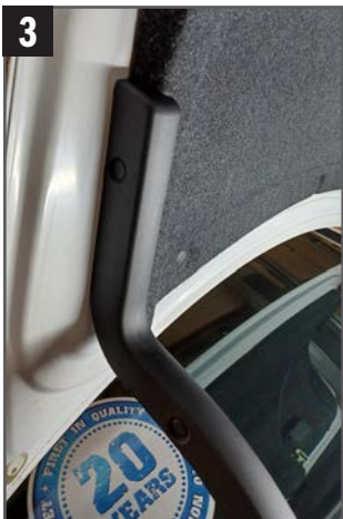
3. Remove the clips/trim from the PS/DS trunk lid support arms.
