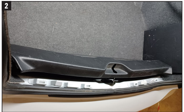
2. Pop loose and remove the trim from the trunks latching point. Tool required: plastic Mold/Trim Remover.
