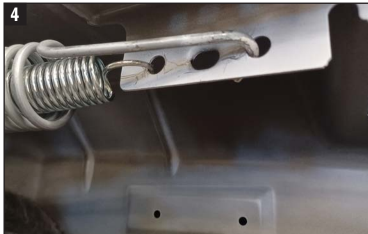
4. Remove any plastic clips holding the carpet sides in place. Gently pull aside exposing the trunk springs. Un-latch the OE spring from its location and place one of the provided springs within it for extra tension. Reconfigure the mounting locations of the OE spring to the most outer hole and the one provided to the rear hole.
