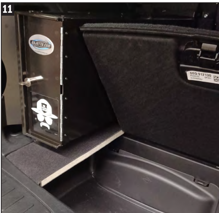
11 Mark lid/cover for cutting in order to gain access to spare tire/jack/etc. Remove lid/cover, cut and replace.
