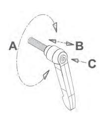
**NOTE:** Insert the ratchet handle through the t side of the articulated swing arm and tighten. Going through threaded side first will not allow the arm to tighten properly
