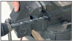
Drill out existing hole to 1/2" or drill new hole per installation instructions.
