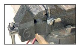
Use %6" box end wrench to secure the flange nut.
