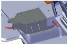
Place GR6 Mounting Plate onto transmission hump. Place Mounting Plate under OEM cover plate, lining up holes to the rear most holes on OEM cover plate. Secure using provided (2) 1/4 x 20 bolts.
