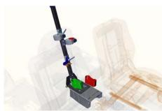
Secure Mounting Plate under rear seat. If OEM wire track (option) was ordered, use OEM bolts from previous removal. If the vehicle does not have OEM wire track (option), use provided tek screws.
