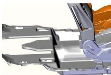
Remove lower rear seat cushion from vehicle by flipping small latches under lip of passenger side/drivers side. If vehicle contains OEM wire track then you will need to remove using 8mm socket.
