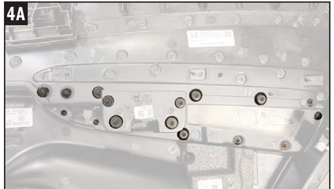
2 Using a trim removal tool, start from the bottom popping loose the Door Panel loose from the frame structure.
