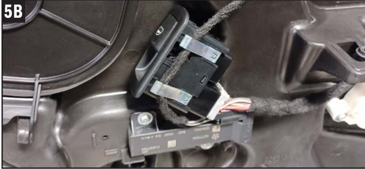
5. Squeeze the tabs while pressing it down to remove the window switch. Once removed secure and tape to the door frame.
