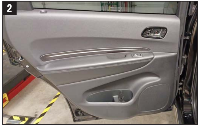
2 Using a trim removal tool, start from the bottom popping loose the Door Panel loose from the frame structure.
