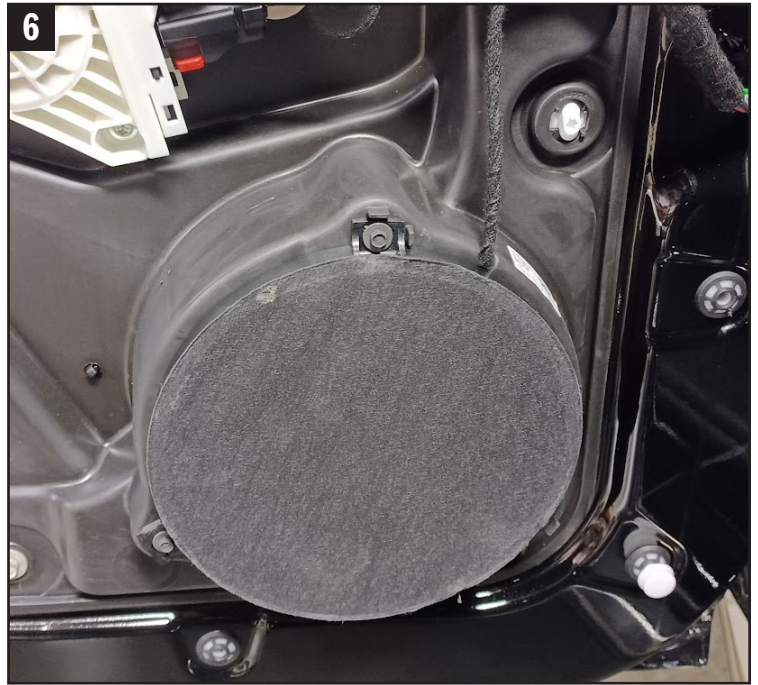
6. Remove the (3) speaker screws. 6 mm Socket. Speaker not reused.
