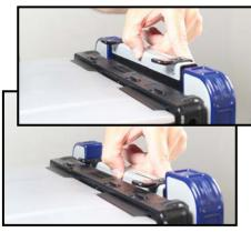
8.) Make any adjustments needed to the Rear Tabs to allow access to any data ports which may have been blocked by the original clamp positions. Loosen the Rear Tab screws (but do not remove) as shown in the image below. Adjust the Rear Tab as needed by sliding side to side in the adjustment tracks. Re-tighten Rear Tab Adjustment Screws.
