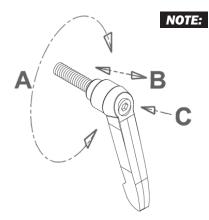
To adjust, tilt pull handle out (B) and rotate counter clockwise (A), release and tighten. If needed, use  $\frac{1}{8}$ " hex head wrench for adjustment (C)
