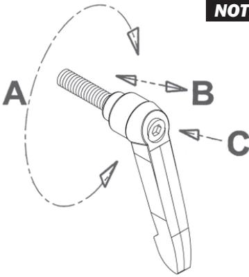
**NOTE:** To adjust, tilt pull handle out (B) and rotate counter clockwise (A), release and tighten. If needed, use  $\frac{1}{8}$ " hex head wrench for adjustment (C)
