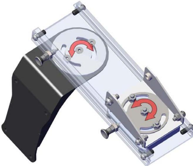
4. The swivel tension to the Motion Arm and Tilt/Swivel Assembly is set at the factory. This can be adjusted by loosening and/or tightening the (3)  $\frac{1}{4}$ "-20 nuts at each location. Use a  $\frac{7}{16}$ " wrench to stabilize the nut and a  $\frac{5}{32}$ " T-handle hex key to turn the bolt.
