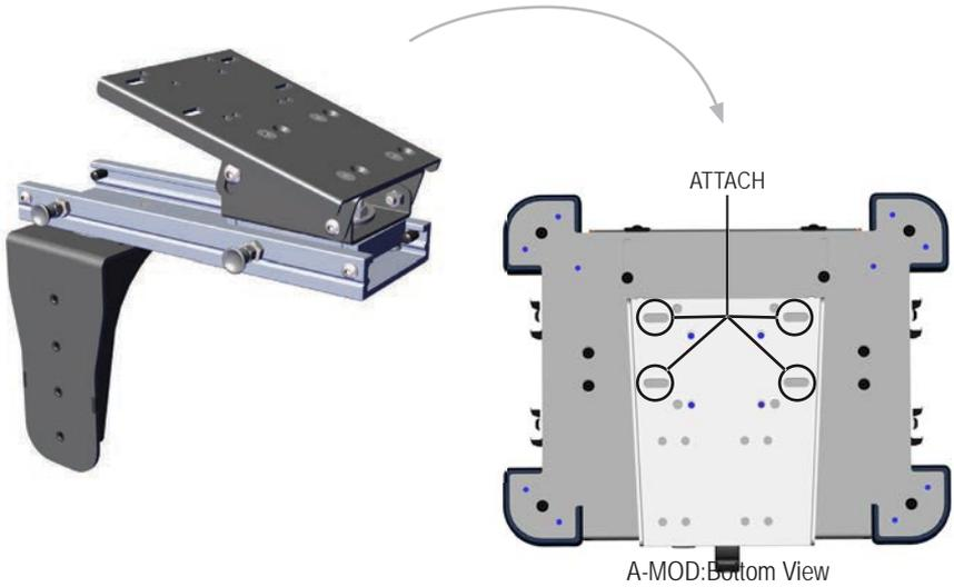
3. Pull the rear knob to release and move the top assembly. Slide it forward to the front locating knob and it will automatically lock in position. From this point you will be able to mount A-MOD Desktop/docking equipment to the top plate via holes and slots from the underside with provided  $\frac{1}{4}$ "-20 bolts and washers.
