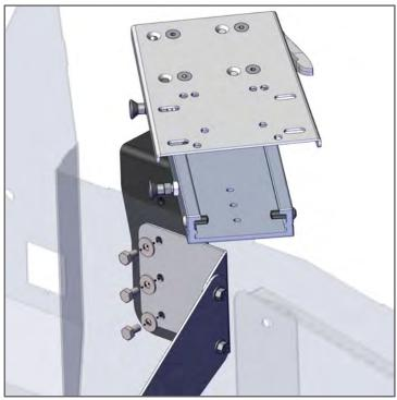
Secure the chosen Mamba Mount to the Console with provided 14' bolts and washers. When secure, go back and fully tighten all previously attached hardware.
