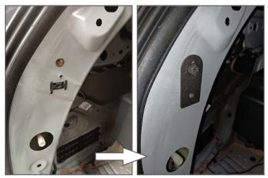
Drill or pop out the OEM mounting clip that held the Jig in place. Install AVK fastener and attach the Driver Side and Passenger Side D-Pillar Straps. Replace OEM trim.
