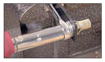
5. Apply pressure on the flange nut, pressing AVK Fastener into hole.
