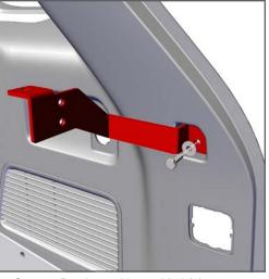
Secure the Driver Side and Passenger Side Front Support Brackets with provided (2) ¼-20 x ¾
