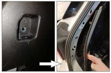
Unscrew the (2) OEM Trunk Cargo Net Tie-Down Hooks and pop loose the D-pillar trim. Drill OEM trim mounting hole to 9/32'.
