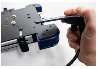
Place keyboard mount on bottom corner, standoff will fit into the diagonal hole where screw was removed.
