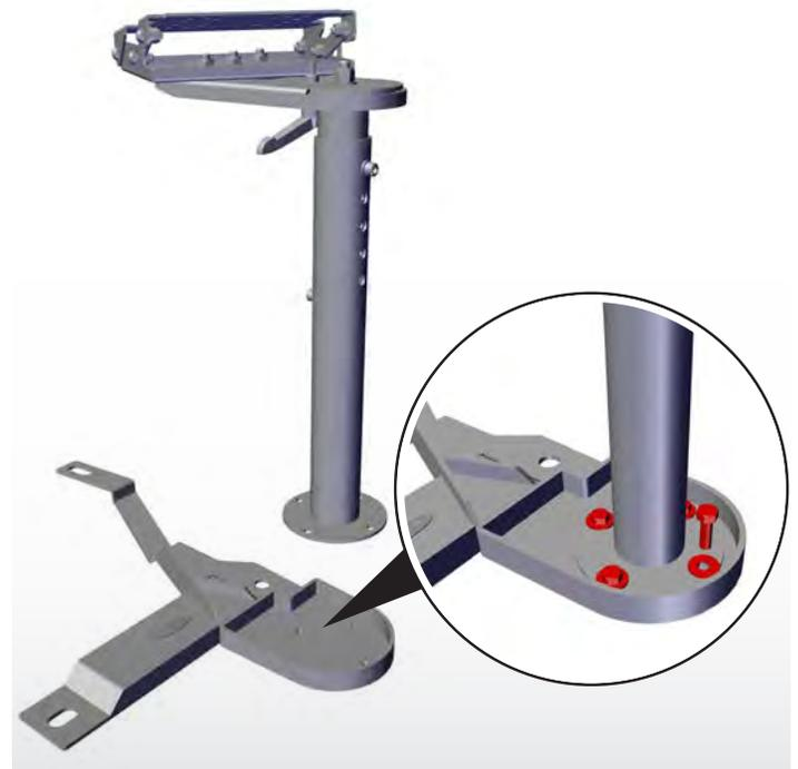
6. Use a 1/2" socket to secure the upright stand assembly to the base with the provided (4) 5/16-18 bolts and washers.
