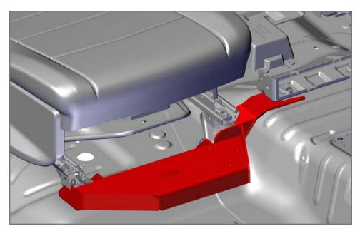
4. Replace the passenger seat back into the vehicle and place the base under the previously removed two front seat bolt locations. Wedge the tab of the HD Base support under the mounting frame of the front middle seat frame and replace previously removed OEM seat bolts securing base in place.
