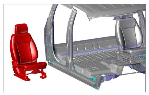
2. Remove the front and rear OEM seat bolts. Tilt the seat back and unplug any electrical connection attaching to the seat. Remove seat from the vehicle.
