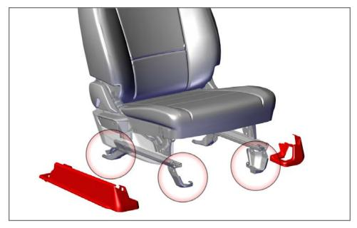
3. Remove the screws and push pin clips on the passenger's seat trim located on door side and front mounting position of the seat. **Note:** *Trim not reused.*
