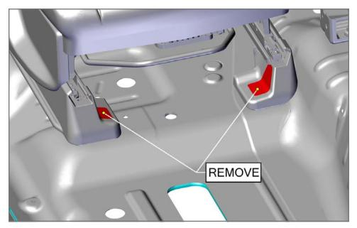
1. Remove the front and rear trim bolt covers using a small flat head screw-driver.
