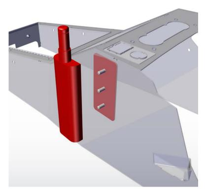
Attach the Backing Plate inside the Console and secure the Side Mount with provided Hex bolts and lock washers.
