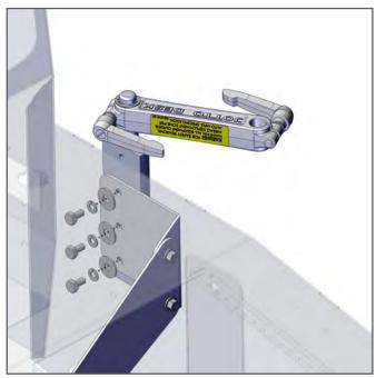
Secure the chosen Console Side Mount to the Console with provided 1/4" bolts and washers. When secure, go back and fully tighten all previously attached hardware.
