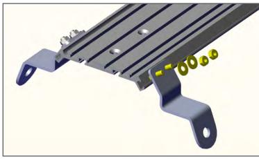
2. Line up the bolts with the holes in each leg and secure with the provided 5/16 washers and 5/16 nuts. Lightly tighten so that adjustment will be easier after installed in the vehicle.
