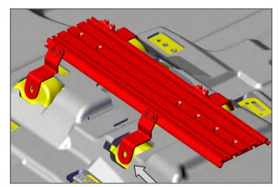
Align the Floor Plate Legs with the holes in floor board. Replace with OEM hardware or provided self-tapping bolts.
