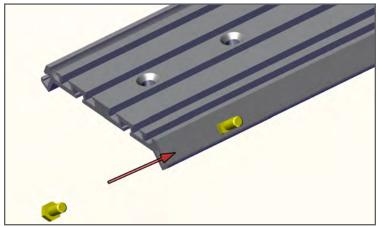
1. Install (8) of the 5/16-18 bolts in the side channel of the Floor Plate, four per side.
