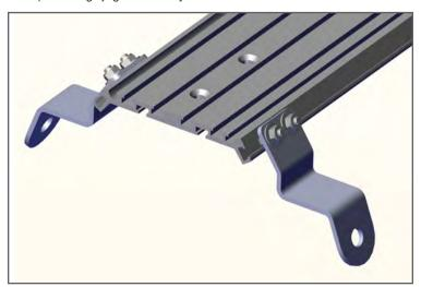
4. Once the Floor Plate is installed, adjust the floor plate (front to rear) as needed. Tighten the 5/16 nuts securing the legs with a  $\frac{1}{2}$ " socket.
