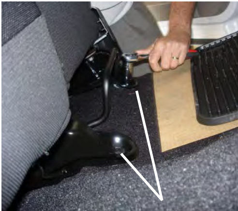
Remove the 2 front seat bolts from the driver side seat.
