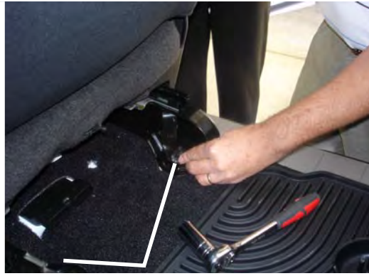
Remove the 2 covers and the two bolts from the rear of the passenger side seat. Remove passenger seat.
