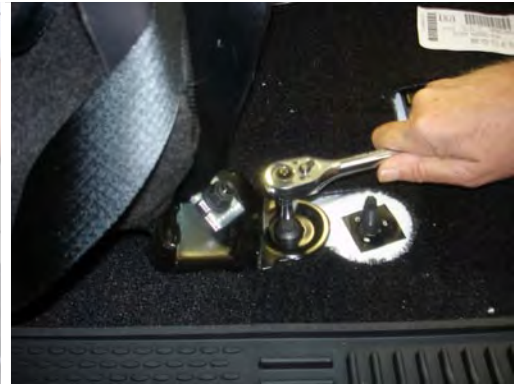
Remove the center console bolt using a T55 Hex Head.
