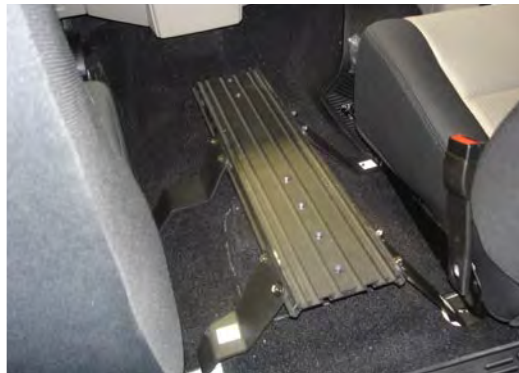
Replace the driver and passenger seats and tighten the bolts reinstalling the seats to secure the floorplate.
