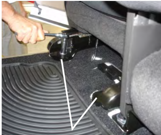
Remove the 2 covers and the two bolts form the rear of the driver side seat. Remove driver seat.
