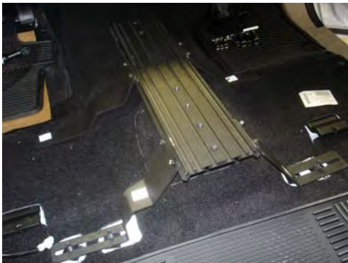
Place the bolts into slots on floorplate now align feet with seat bolts and align bolts to holes on feet and tighten nuts.
