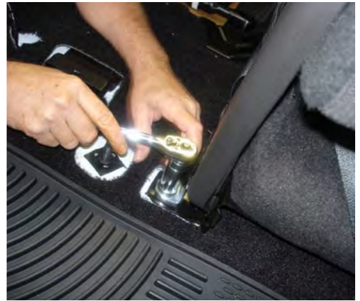
Remove the center console bolt and now remove console.
