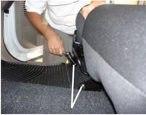
Remove the 2 front seat bolts from the passenger side seat.
