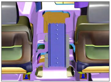
2. After removing OEM seat section, locate and wiring to prevent issues. Place Floor Plate on top of transmission tunnel and position as desired.
