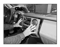
Once the clip is started into place. Then push OEM console back into the original position with an upward and forward motion.
