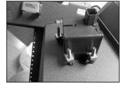
Attach airbag on/off switch. We suggest using (3) 10-24 x 1.5 screws and (3) 10-24 nuts.
