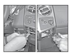
Remove the screws from the left and right side behind the corner panels.
