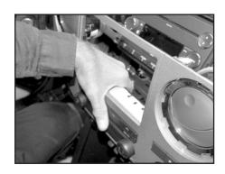
Setting the OEM upper dash trim back into position. Reach through the radio opening and press down on the metal clip of the OEM brake controller.
