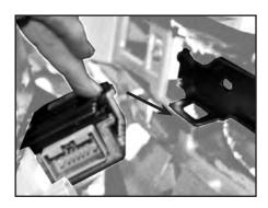
Slide OEM upper dash trim into place. Make sure the clip goes under the OEM dash frame as shown.
