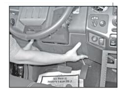
Replace the screw on the left side of the console and replace the panel under the steering column.
