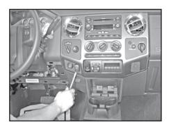
Use a flat head screwdriver to remove the left and right corners of the dash.
