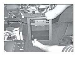
Shift console into place. Be sure outer holes line up (see pic). Now tighten down all four screws from step 14 and 15.
