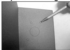
Using a punch knock out all 4 stamped holes on drivers side of console.
