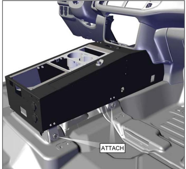
2. Outside of vehicle, loosely attach Rear Legs, Front P/S, and Front D/S Legs with provided hardware. Install Contour Console into the vehicle from the rear seat area, sliding forward until mating up with OEM dash structure.
