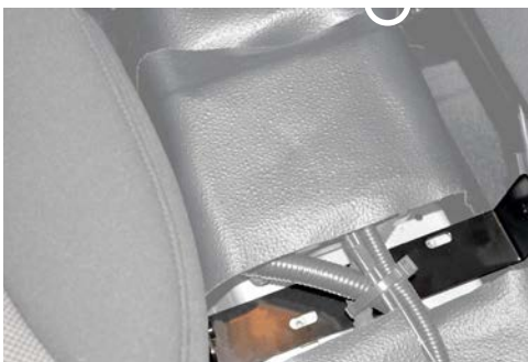
Slide Rear Mount Plate under OEM wiring and replace OEM cover plate. Secure using the supplied all thread studs.
