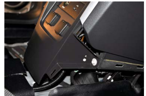
Remove (2) OEM Trim Panels from Side of Dash
