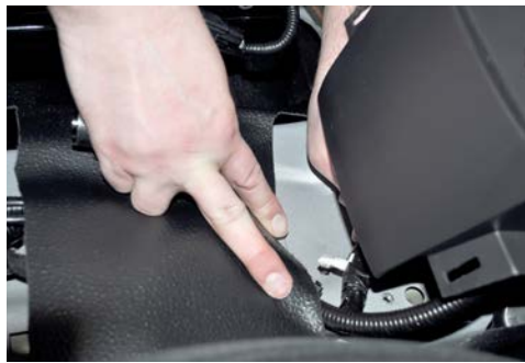
At dash of OEM cover plate – remove tab that secures a cable to OEM cover plate
