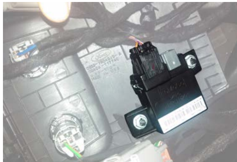
At dash of OEM cover plate – remove tab that secures a cable to OEM cover plate
