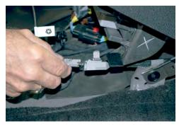
Disconnect wiring harness for 12V and USB from OEM console.
