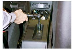
This will expose the plastic OEM console. Remove (1) 10 mm flange nut from center of plastic console. Nut will be re-used.
