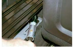
Remove (2) 8mm mounting screws at the rear mounting point of the aluminum floorplate. Screws will be re-used. This will allow the removal of the OEM aluminum floorplate and brackets.
