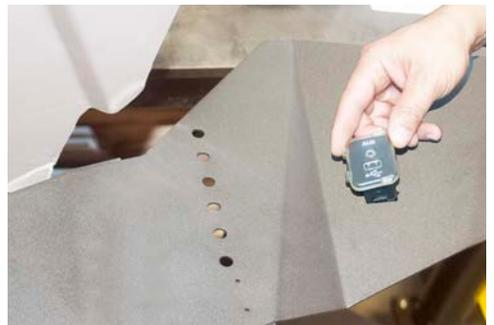
Utilize the provided USB extension cable. Plug the male end into the harness under the dash and the female end into the USB connector. Re-mount USB connector into P/S front section.
