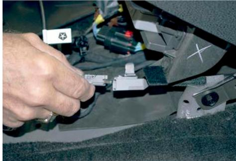
Disconnect wiring harness for 12V and USB from OEM console.
