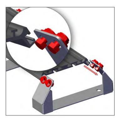
3. Lightly secure (8) of the 5/16-18 bolts, washers and nuts to the Floor Plate Brackets. Slide the Floor Plate in from the rear, aligning the bolts with the sides grooves on the Floor Plate sides.
