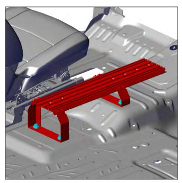
4. Place the Floor Plate in desired location by sliding forward and back. Secure by tightening the 5/16 nuts.
