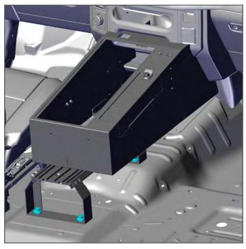
6. Place Console on Floor Plate making sure the front and sides are up against the dash and secure in place with provided (4) 5/16-18 bolts, washers and nuts. Plug in the OEM USB Cable(s).
