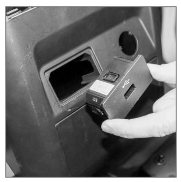
5. Using a trim tool, pop out and relocate the USB from the vehicles dash to the top of the Contour Console.
