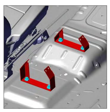
2. Place front and rear Floor Plate Brackets over hole locations. Secure with provided bolts or OEM hardware.
