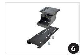
Outside of vehicle insert 4 carriage bolts through bottom of plate. Align console slots onto carriage bolts and finger tighten with provided nuts.
