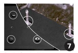
Position floorplate/AK-7 onto transmission hump. Aligning the holes of the bracket with the OEM mounting studs. Tighten bolts and flange nuts.
