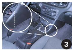
Mark and cut OEM console for best placement of console.
