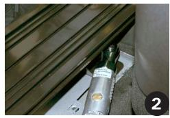
Remove (2) 8mm mounting screws at the rear mounting point of the aluminum floorplate. Screws will be re-used. This will allow the removal of the OEM aluminum floorplate and brackets.
