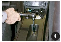
Remove (1) 10 mm flange nut from center of plastic console. Nut will be re-used. Remove the cut OEM console piece.
