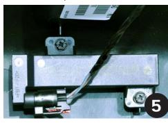
Remove Ignition Proximity Sensor from plastic OEM console. Ignition Proximity Sensor should be remounted onto top of transmission hump with Velcro or double sided tape.
