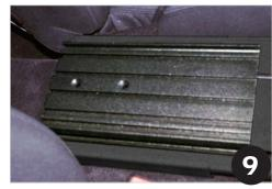
Position 12" extruded floorplate onto floorplate/AK-7 and secure using pan head bolts.
