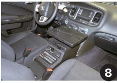
Position Jotto Desk AK-7 Console into desired position and fully secure bolts with nuts
