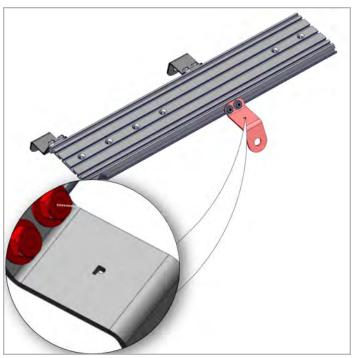
Line up the bolts with the holes in each leg and secure with provided 5/16 washers and 5/16 nuts. NOTE: Indicate the correct leg for the passenger front with the cut out "P".
