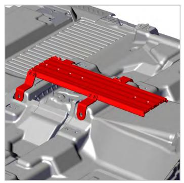
4. Secure the Floor Plate Legs to the OEM mounting holes with provided hardware. Once installed, adjust the Floor Plate (front to rear) as needed. Tighten the 5/16 nuts securing the floor plate in position.
