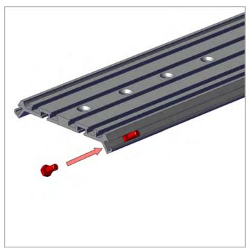
Install (8) of the 5/16-18 bolts in the side channel of the Floor Plate, four per side.
