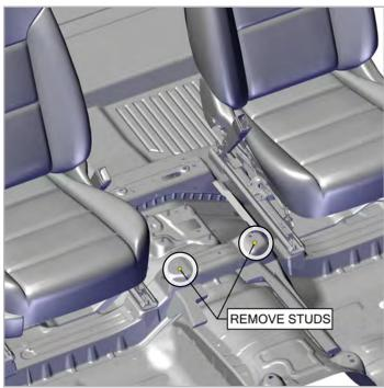
Some vehicle OME trim levels may have (2) threaded studs located on top of
