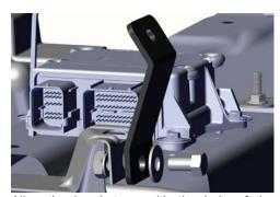
Align the bracket up with the hole of the metal flange that protrudes from the center transmission hump. Insert the 5/16-18 bolt through the washer and secure it with the provided 5/16 nut.
