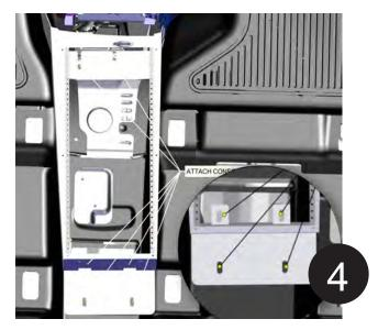
Secure top of console by using (2) M6-1.0 hex flange nuts. Secure bottom of console with (2)  $\frac{1}{4}$ " washers and  $\frac{1}{4}$  self-tapping screws.
