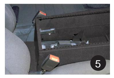
Relocate the Proximity Sensor to the mounting studs on the Jotto Desk Contour Console. Use the provided 8-32 nylon washers and place between console and sensor.
