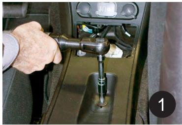
Remove forward OEM console plastic cover, then remove (1) 10 mm flange nut from center of plastic console. Nut will be re-used.
