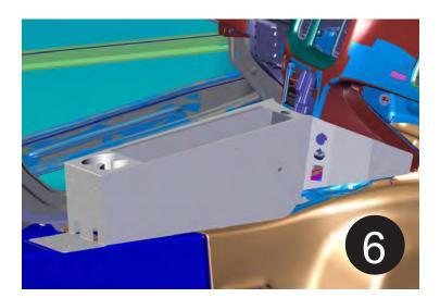
Console can now be adjusted forward and up to ensure a tight fit/finish with the OEM dash structure.
