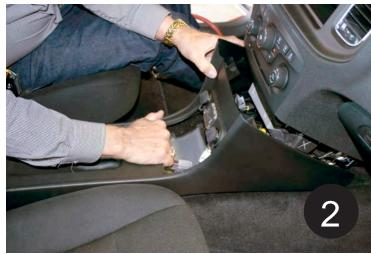
With both hands, grasp the plastic OEM console on both sides and pull directly rearward to release.
