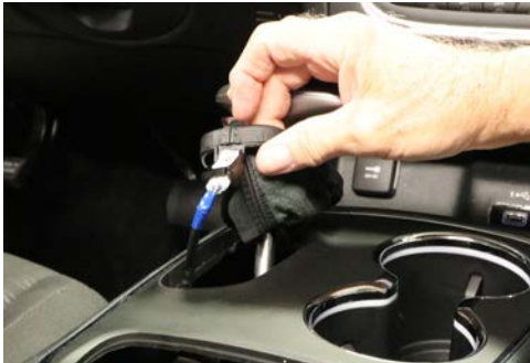
Pop up shifter boot. Unscrew bolt on shifter with T20 bit and unplug wire cord.
