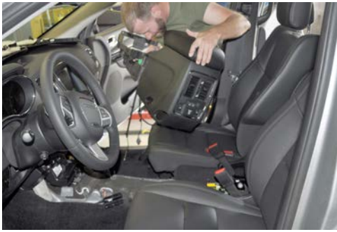
Remove OEM console from vehicle.
