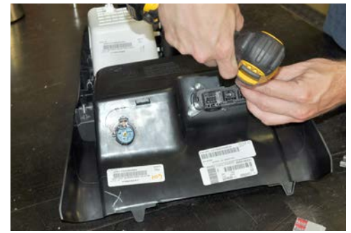
Using a T20 bit, remove (4) screws and set aside media component to remount into Contour Console.
