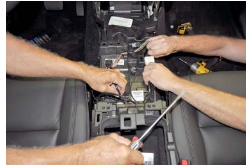
Disconnect wiring harnesses and harness clips.
