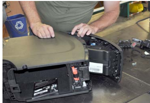
Now pry rear OEM cover from console.
