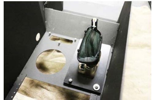
With the console turned over, install the boot and shifter and re-tighten T-20 screws. Snap the boot clips into the Filler Plate.
