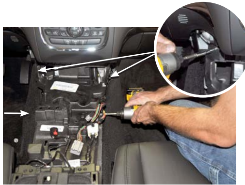
Remove (2) 10mm bolts and (2) 7mm bolts.
