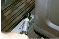
Remove (2) 8mm mounting screws at the rear mounting point of the aluminum floorplate. Screws will be re-used. This will allow the removal of the OEM aluminum floorplate and brackets.
