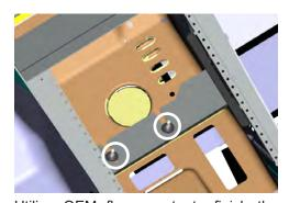
Utilize OEM flange nuts to finish the installation of Jotto Desk Contour Console, securing onto OEM mounting studs. This will snug up the console to the OEM dash.
