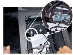
Remove 10mm OEM nuts from studs near proximity sensor. Pull up rubber pad placing front mounting bracket under pad. Replace rubber pad and proximity sensor and secure using OEM nuts.
