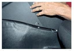
Secure front mounting bracket to D/S of console using provided 10-32 socket head cap screw.
