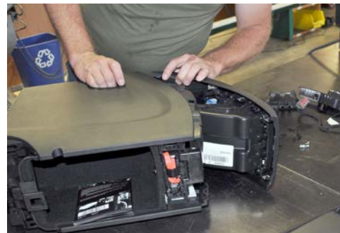
Now pry rear OEM cover from console.
