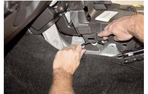
On the driver side of center console, unsnap Manual Park Release cable from OEM substructure.
