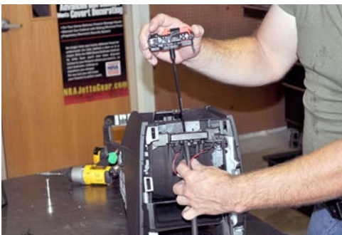
Remove Duct. Using a flat head screwdriver, pop out clips holding cable in place. Then pull cable through, and remove cable clips. Set aside Manual Park Release to be reinstalled into the Contour Console.
