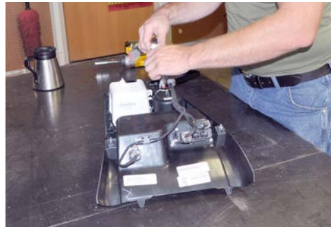
With OEM console out of vehicle, begin to remove all components from console. First, remove media wire harness.
