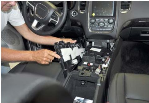
Pop off front left/right side panels from OEM console.
