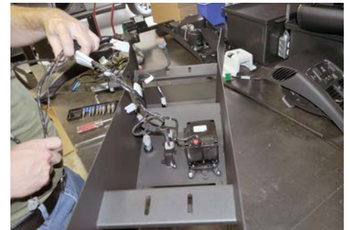
Reinstall components back into Jotto Desk Contour Console using the same hardware from OEM console.
