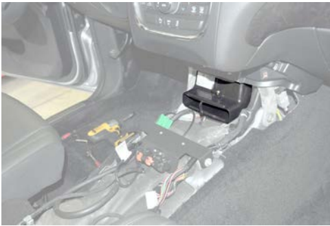
Install foam insert into open duct.
