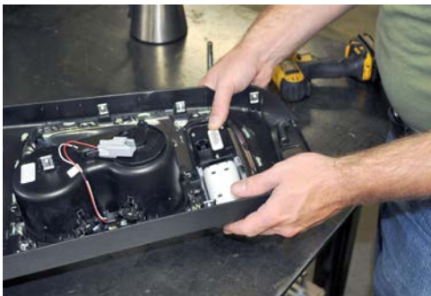
Traction switch/coin tray will pop out from underside of OEM console. Set aside.
