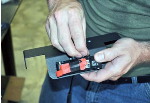
Using 5/16" hex head bolts, attach Manual Park Release to Forward Mount Bracket.
