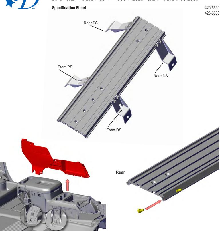
Unsnap side trim from left and right of center console exposing center console OEM bolts. Remove center console.
