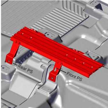
Line up the bolts with the holes in each leg and secure with the provided 5/16 washers and 5/16 nuts. Lightly tighten so that adjustment will be easier after installed in the vehicle.
