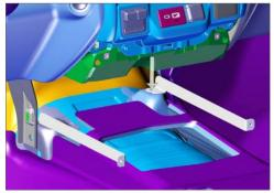
3. Attach the Lower Left and Lower Right Support Brackets to the OEM studs located by the main center dash supports. Loosely secure with provided flange nuts.
