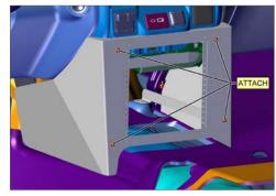
5. Place the Console into the vehicle. Secure in place by attaching the (4) provided screws through the front of the console and attaching to the previously installed Lower and Upper Brackets. Tighten flange nuts on Lower Support Brackets to complete installation.
