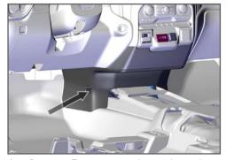
.. Remove 7 mm screw located on the driver side lower trim.
