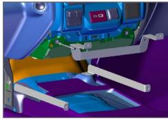
4. Attach the Upper Bracket to the dash with provided M4.2 x 1.41 x 2.0 screws. Tighten into place.
