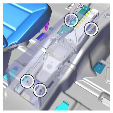
1. Remove the factory front and rear OEM 10 mm nuts holding the OEM Cover Plate in place.
