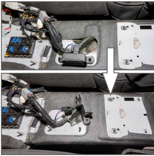
4. Remove and unplug the Proximity Sensor using 10 mm socket.
