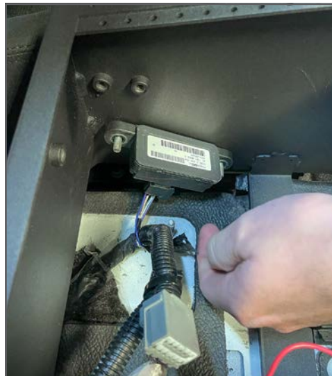
10. Plug in and relocate the Proximity Sensor to the mounting studs in the Console with previously removed OEM flange nuts. You can now relocate the OEM 12v outlets and plug in OEM harness.
