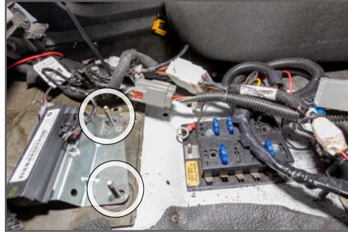
5. Disconnect the main OEM harness and loosen/remove OEM flange nuts holding OEM sensor plate in place.
