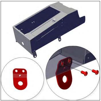
2. Outside of vehicle, loosely attach Rear Legs, Front P/S, and Front D/S Legs with provided hardware. Install Contour Console into the vehicle from the rear seat area, sliding forward until matching up with OEM dash structure.
