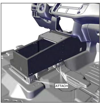
Adjust Mounting Legs as needed - to position over OEM mounting points and tighten legs to Contour Console. Secure Mounting Legs to OEM Substructure using OEM 12 mm bolts or provided 1/2" - 13 x 1.5 TCS Bolts.
