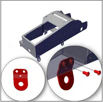
Outside of vehicle, loosely attach Rear Legs, Front P/S, and Front D/S Legs with provided hardware. Install Contour Console into the vehicle from the rear seat area, sliding forward until matching up with OEM dash structure. NOTE: Indicate the correct leg for the passenger front with the cut out "P".
