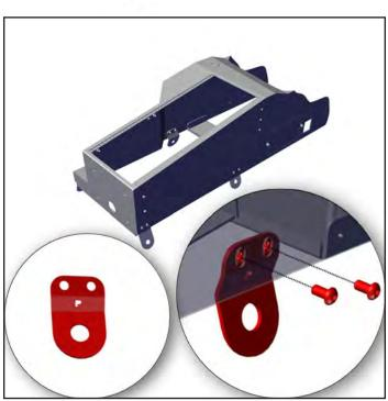
Outside of vehicle, loosely attach Rear Legs, Front P/S, and Front D/S Legs with provided hardware. Install Contour Console into the vehicle from the rear seat area, sliding forward until matching up with OEM dash structure. NOTE: Indicate the correct leg for the passenger front with the cut out "P".
