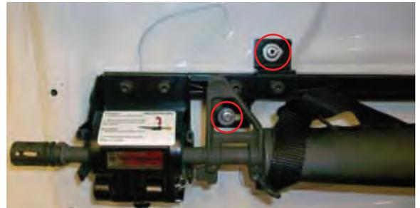
Secure with 2 rivets on each side
