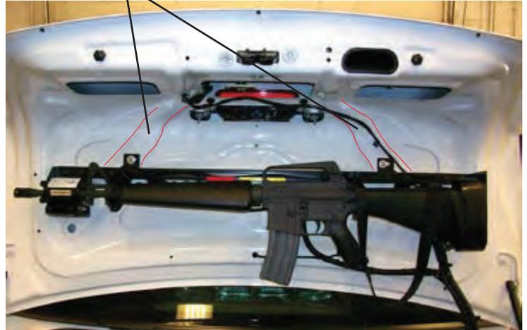
1. Secure weapon in gun rack, then position weapon mount in desired location. Slide adjustable "Z" brackets to meet up with the raised contours of the trunk lid, as shown in picture A.
