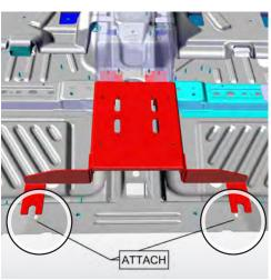
Attach the rear left and right legs of the Mounting Base to the underside of the rear seat with OEM hardware.
