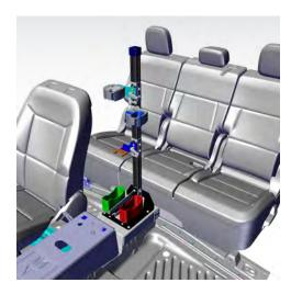
Attach Backbone assembly to top of Mounting Base using (4) provided 1/4" x 20 x 3/4" button head cap screws
