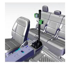
Attach Backbone assembly to top of Mounting Base using (4) provided 1/4" x 20 x 3/4" button head cap screws
